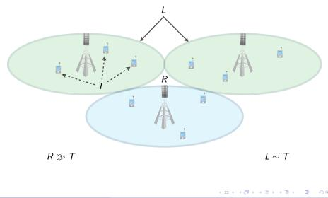
For T transmit antennas and R receive antennas, even for a static channel, RT channel coefficients must be estimated.
