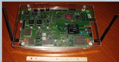
1998: 1 st Small Cell based on The US Digital Cellular Standard IS-136 – AT&T Bell Labs
